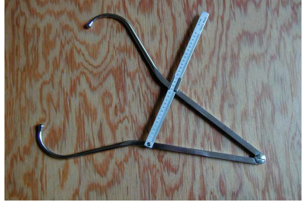
FIGURE 3 Spreading Caliper
