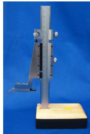
FIGURE 11 Modified Height Gauge
