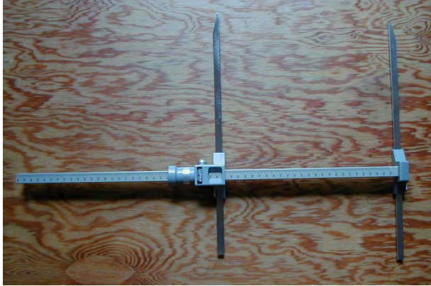
FIGURE 2 Beam Caliper
