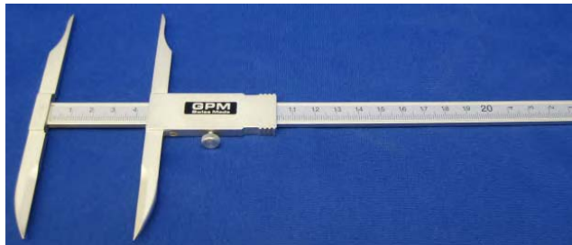
FIGURE 4 Sliding Caliper
