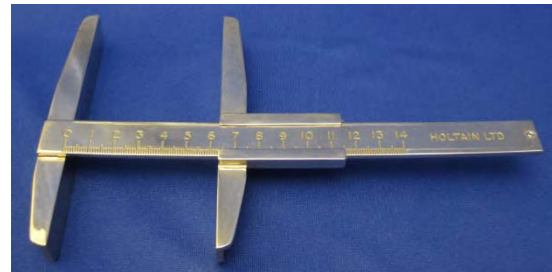
FIGURE 5 Holtain Caliper
