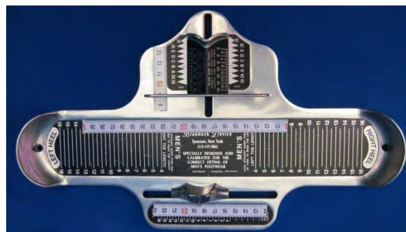
FIGURE D-10 Modified Brannock Device
